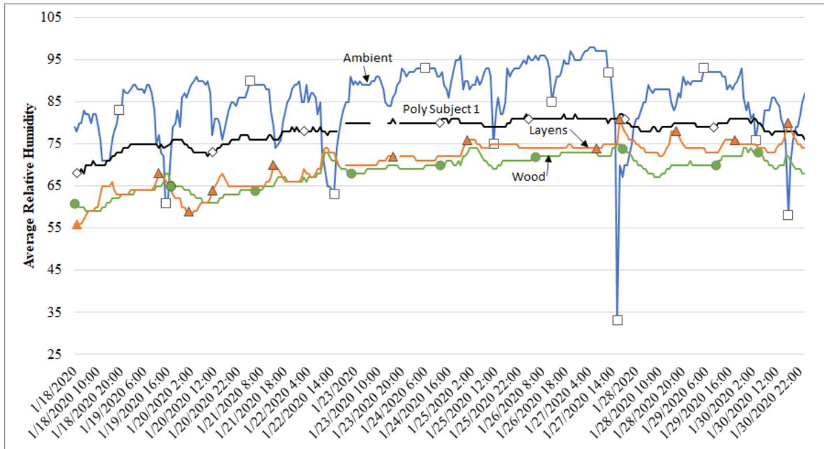
**Figure 7.** Comparison of Relative Humidity levels. The relative humidity is higher in the Poly because the average temperature is 10 degrees warmer than the Wooden hives. As temperature increases, relative humidity increases.
