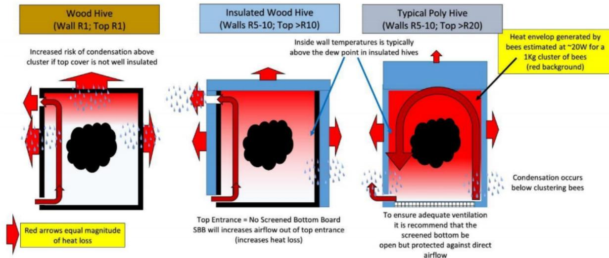
**Figure 3.** How Insulation Works (Tardif, 2020).
