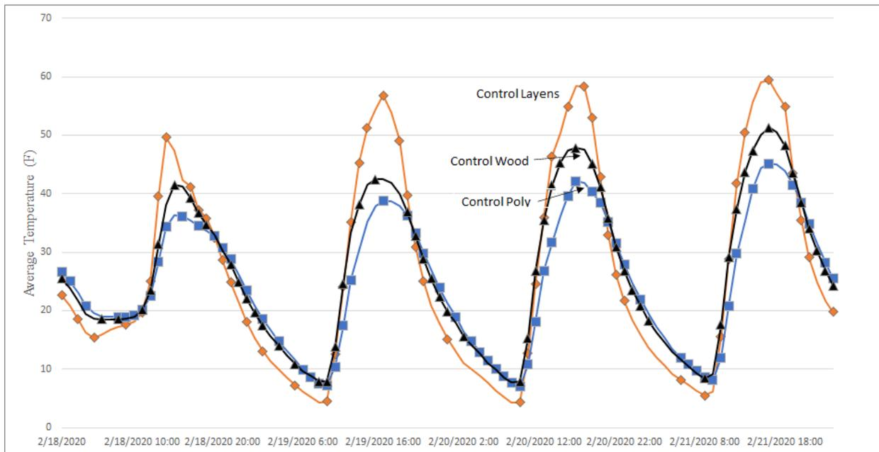
**Figure 4.** Fluctuations of temperature in empty Control Hives.
